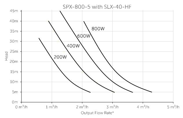
\* Chart reflects real-world Impact Pump data at 25°C water temperature, including losses from 40mm PN16 HDPE pipes. Performance data published by electric submersible-pump manufacturers should be corrected for pipe-flow friction and cable losses (not normally included) for comparison. These losses often reduce wire to water efficiencies by 5% or more.
